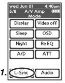
2. Select the time lag with the ◀ and ▶ cursor buttons on the remote control unit.
